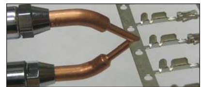
Tack welding of carrier strip
